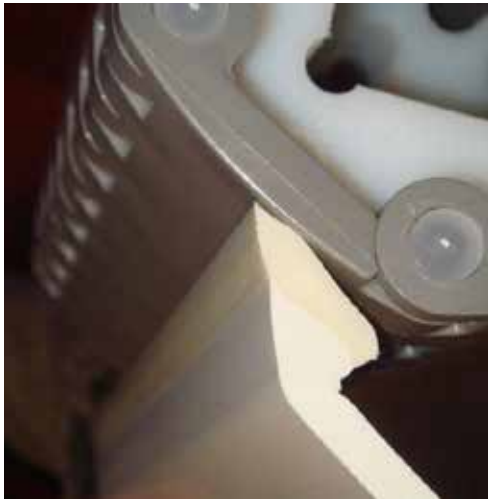
The soft scraper blade is shown here pressed against a curved-top modular belt.
