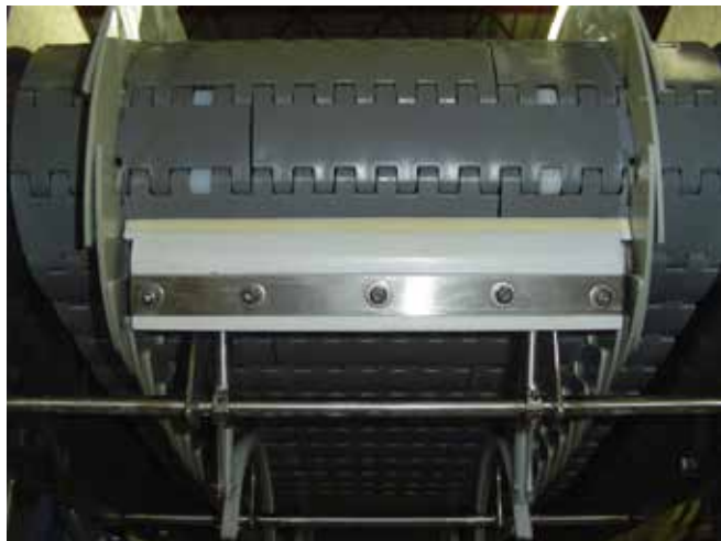
The scraper can be installed as illustrated under the conveyor onto the existing conveyor frame.
