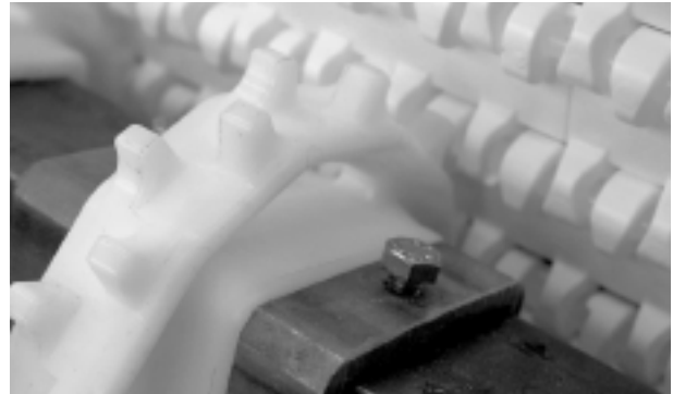
Curved faces of teeth engage on hinge (link-eyes).
