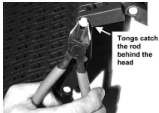
Optional: Extract the rod using a side cutter.
