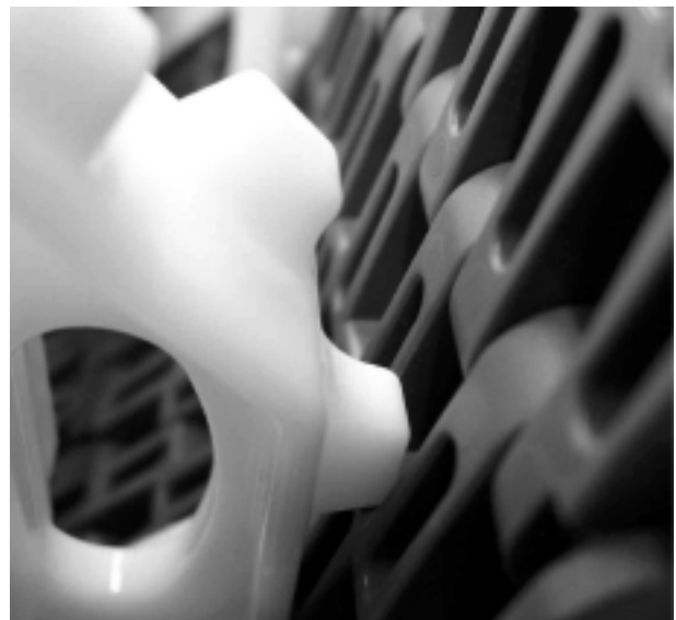
Straight teeth faces on cross rib, curved faces on round link ends.
