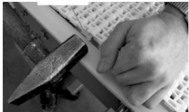
Gently tap its head into retaining position.
