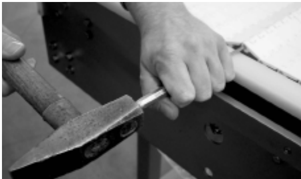
Punch rod out of retaining head by striking the rod end opposite to retaining head.
