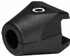
Rod end clamp for guide rail is supplied in polyamide with stainless steel hardware. (fits guide rail with «S» = 0.06" or 0.08")
